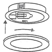
Fit locking cams of diffuser ring into the openings of the housing and turn them clockwise until it stops
