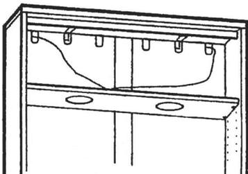
To access the wall fixing brackets, take out the four brass shelf supports and lower the lighting shelf to reveal the sliding fixing plates inside the top of the cabinet.
