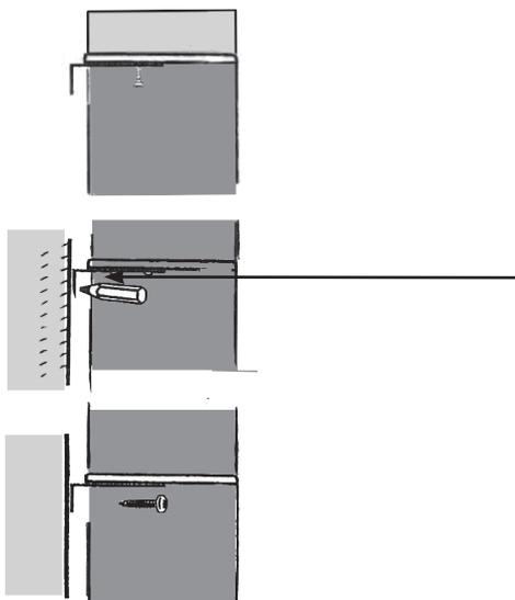
Mark the wall with a pencil through the hole in the fixing plate
