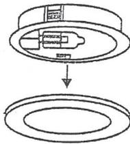
Carefully pull diffuser ring with glass out of the spotlight housing
