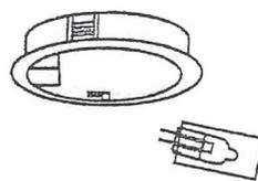
Remove the spent lamp and replace it with a new G4 halogen lamp (10W) only. Do not touch bulb with our fingers but use a cloth or paper.
