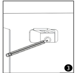
Then remove the unit from the wall so that the marked holes can be drilled. Ensure you use an appropriate fixing type for your wall (see page 5). Then return the unit to position.
