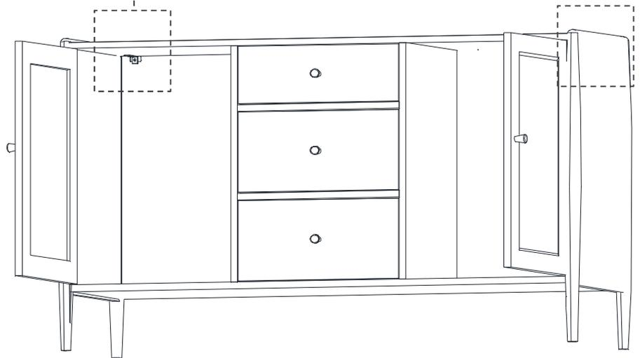
4 Secure the unit to the wall fixings with screws through the brackets.
