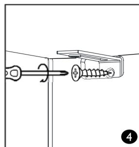
5 Finally add an extra securing screw to the hole in the long face of the brackets.
