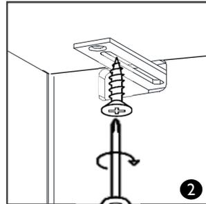
3 Mark the wall for drilling through the hole in the short face of the bracket.
