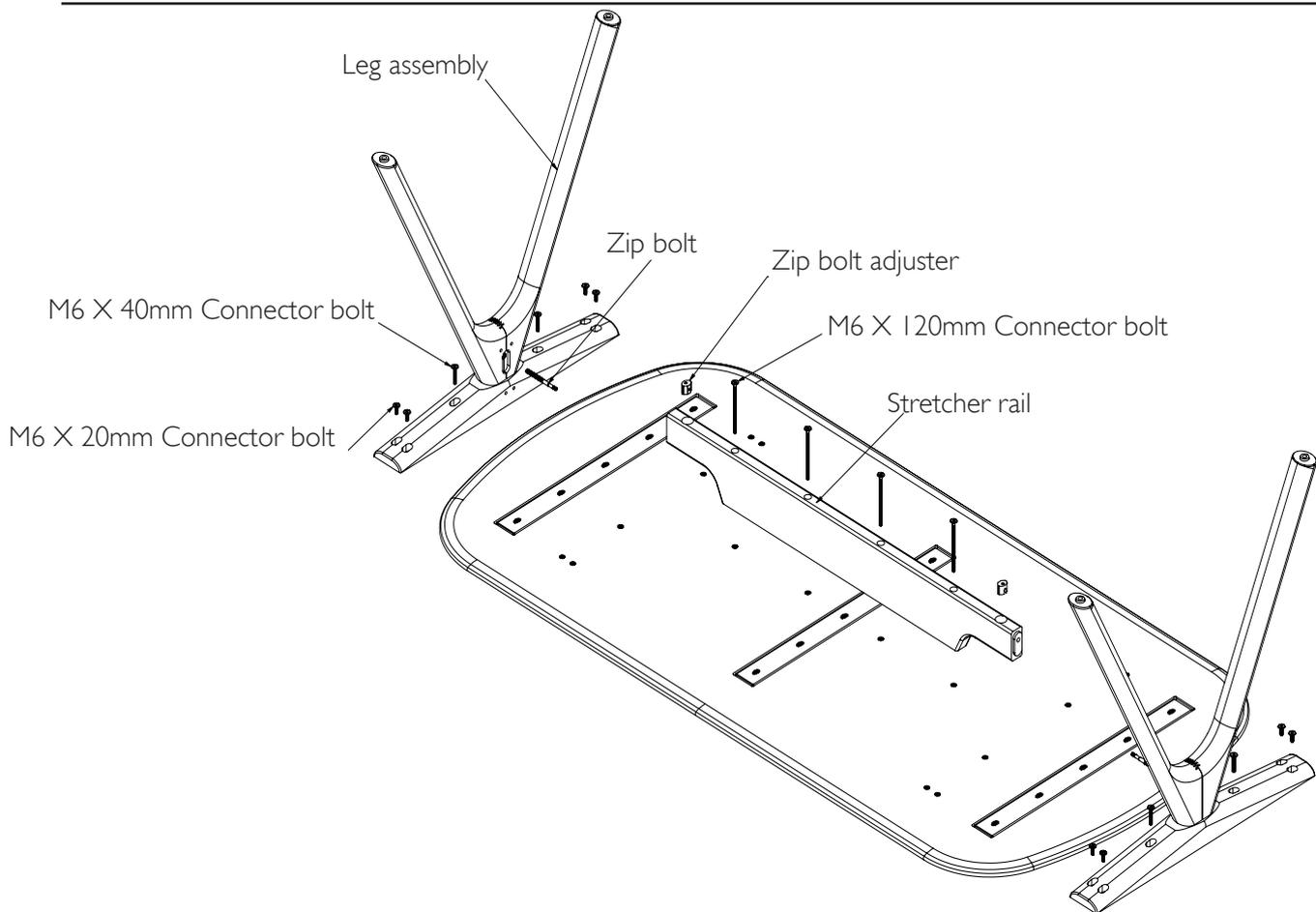
1. Fit the zip bolt (E) into the leg assembly, turning anti-clockwise. Once secured locate the zip bolt (E) into the hole in the end of the stretcher rail. Place the zip bolt adjuster (D) into the circular recess in the stretcher rail.
