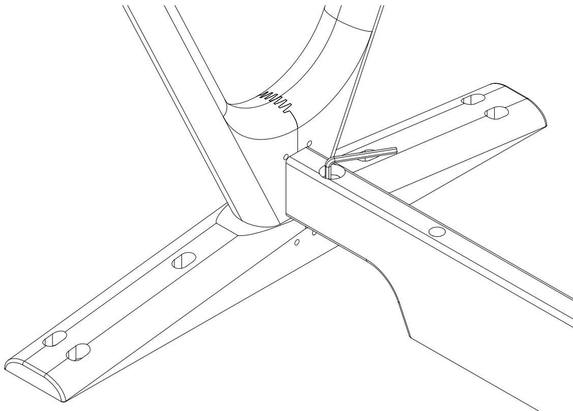
3. Once the underframe is assembled, secure to the underside of the table top. Fasten with the relevant connector bolts using the 4mm Allen key (G).
