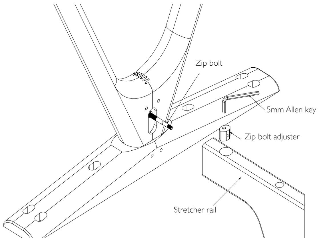
2. Secure the fitting by turning the socket in the zip bolter adjuster (D) clockwise with the 5mm Allen key (F), Fasten until hand tight.
