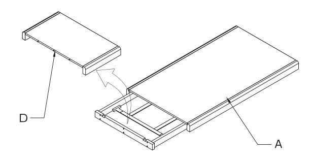
2. Two people may be necessary to carefully turn the table top face down onto a smooth soft surface such as carpet. Put the leg frame B/C to the table top and matching the holes, secure the bolts and washers (locking washer first) FINGER TIGHT ONLY into the legs through the holes on the end rail of the table top.
