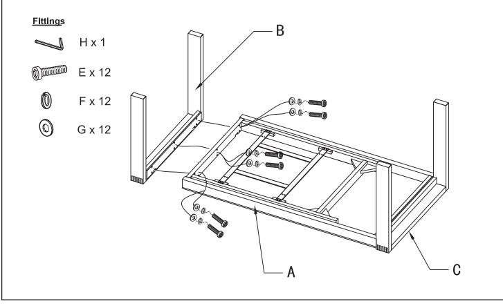
3. CAUTION this table is very heavy. With the aid of another person carefully lift the table and turn it over, taking care not to turn the table over on two legs as this may cause damage.
