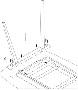
3. Using the allen key (B) fix 8 bolts. Repeat with the other side.
