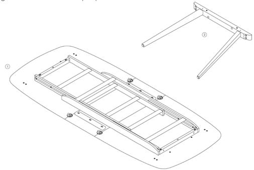
2. Take one leg assembly and aligning the 8 bolts and holes as shown below.
