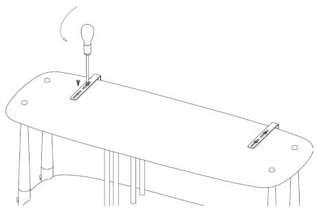
2. Turn the brackets around so the flange is pointing up and reattach the using the screws keeping them slightly loose. Slide the brackets along the slot until it meets the wall. Tighten the screws.
