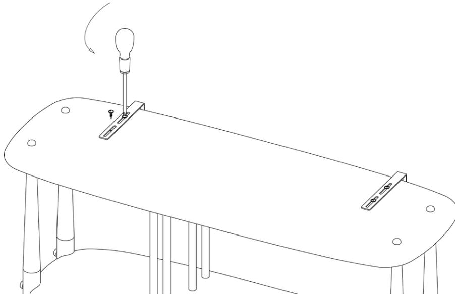
2. Turn the brackets around so the flange is pointing up and reattach using the screws keeping them slightly loose. Slide the brackets along the slot until it meets the wall. Tighten the screws.
