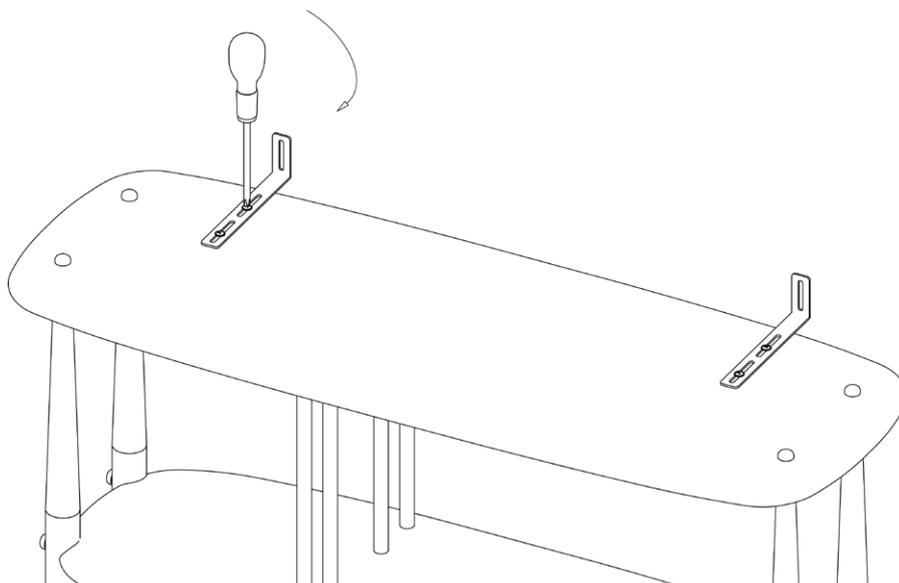
3. Using suitable fixings (not included) affix to the wall.
