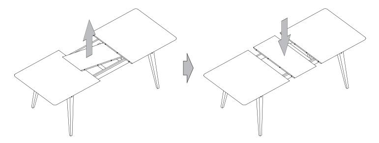
7. Fix the top panel in place using the catch locks.
