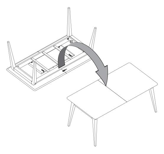
5. Release the two catch locks under the top panel and extend both halves.
