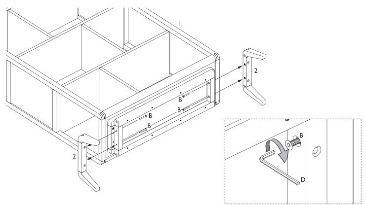
3. Fix the remaining 4 allen head bolts (B) to the legs (2) by using the allen key (D).
