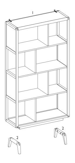
I. Insert 4x wooden dowels (A) into the pre-drilled holes under the shelving unit (1) by using a soft hammer.
