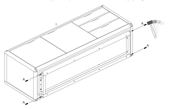
I. Insert 4x wooden dowels (A) into the pre-drilled holes under the cabinet (I) by using a soft hammer.
