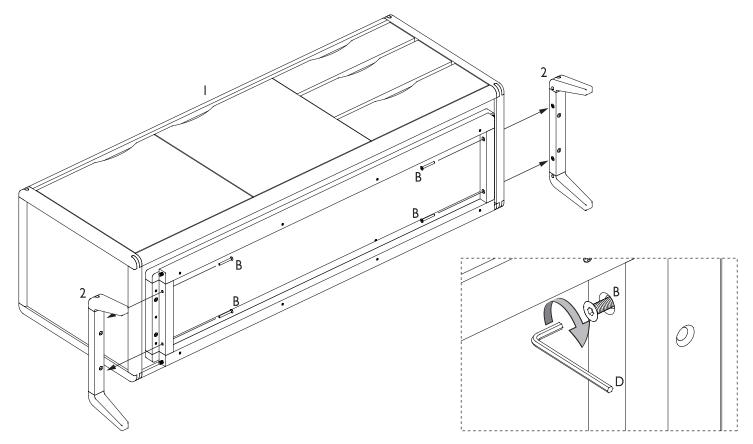
3. Fix the remaining 4 allen head bolts (B) to the legs (2) by using the allen key (D).
