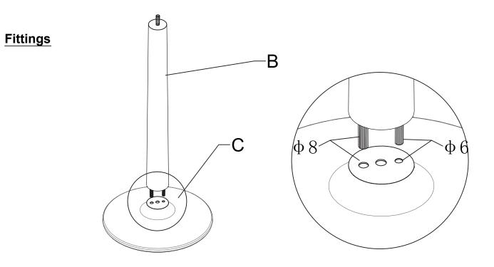
2. Use the allen key(D) to fix the the 65mm bolt (E) onto the base panel C as shown below. Tighten the bolt to make sure they are held in place well.
