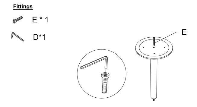
Attach the top panel (A) onto the column (B) using the pre-drilled bolt in the column. Twist the top panel onto the column until they are securely connected. Please see the illustration below.
