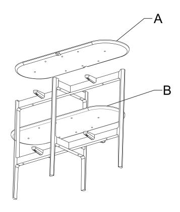
4. Using the M5 Allen key (G) to fix the 8pcs 8\*50mm bolts (H) to the shelf panel (B) and top panel (A) via the predrilled holes on the cross rails (E).
