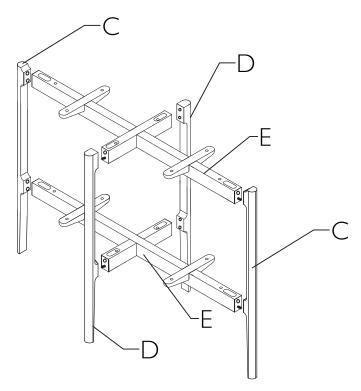
2. Using the M4 Allen key (F) to fix the 8pcs 6\*45mm bolts (I) and 8pcs half moon washer (J) on the legs and cross rails so that they are completely immobilized as shown below.
