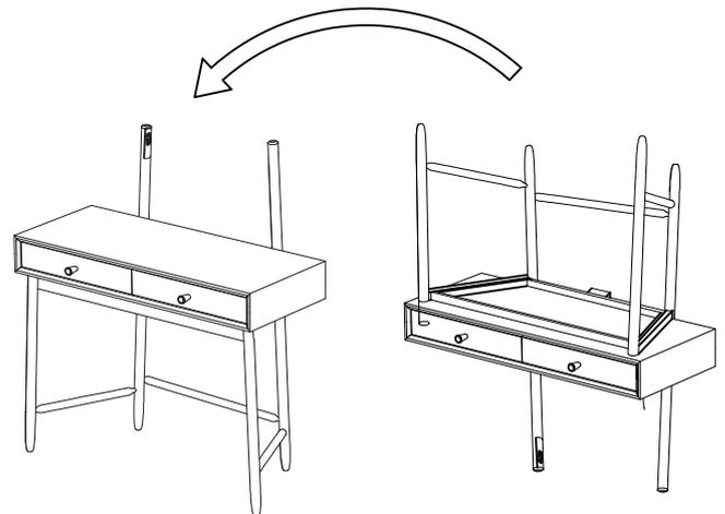
2. Attach the left leg (B) and right leg (C) onto the back side of the drawer box unit (A) using 2pcs M6\*30 bolt (F) as shown below.
