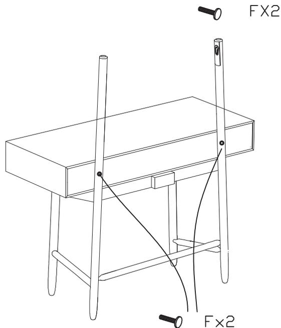
3. Put the mirror(E) onto the left & right legs (B&C) as shown below.
