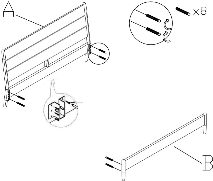
2. Making sure the holes in the side rails (C) are facing upwards, AND that you have the Left and Right rails, (see page 2) on the correct sides, locate the side rails onto the protruding threads on the headboard and foot board. As you do this, slide a half moon washer onto the thread when it comes through into the circular hole in the side of the rail, then screw on one of the 8 nuts FINGER TIGHT ONLY. Repeat with the other 3 corners. then TIGHTEN FIRMLY WHEN ALL FOUR CORNERS ARE SECURED.
