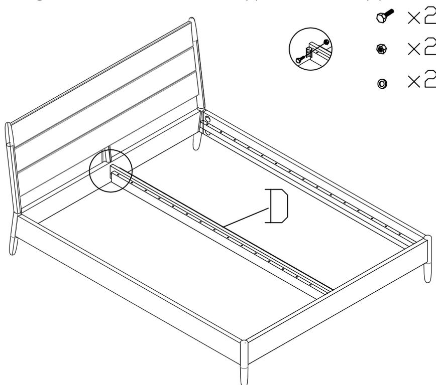
4. Push a plastic cap onto the end of each slat, ensuring that the peg is facing downwards, push the slat into the pre-drilled holes as shown below. Repeat for all of the slats. Assembly is then complete.
