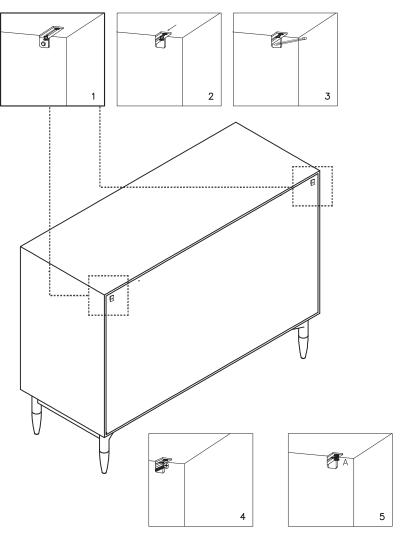
5. Final tighten up the wall fixings using the provided screw as figure 5 shown.
