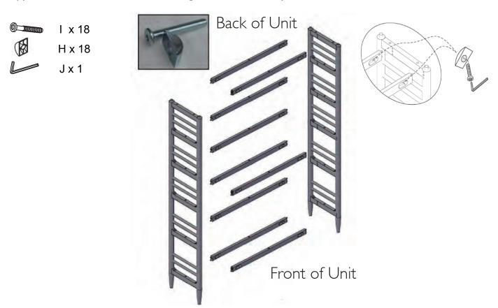
Using 21pcs bolt to fix the 5pcs shelf panles onto the shelf support rails and top panel onto the side frame and top shelf support rail. Tighten with allen key as shown below.
