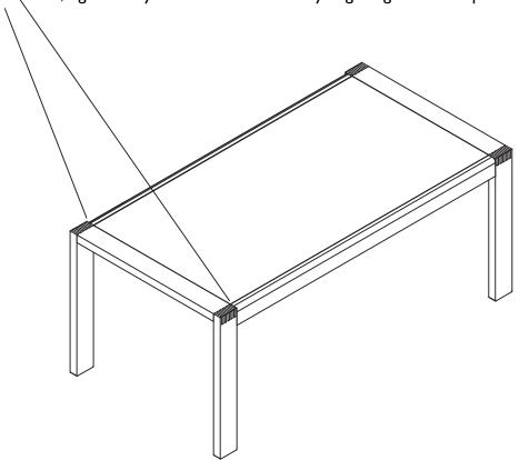
4. Pull the left leg frame outwards as shown, and locate the extension leaf in place. Push the left leg frame back together and secure in place using the two metal clips underneath the side of extension leaf and two metal clips underneath the side of table top. Do the reverse to close the table. Note the extension leaf can be stored FACE DOWN on the frame underneath the table.
