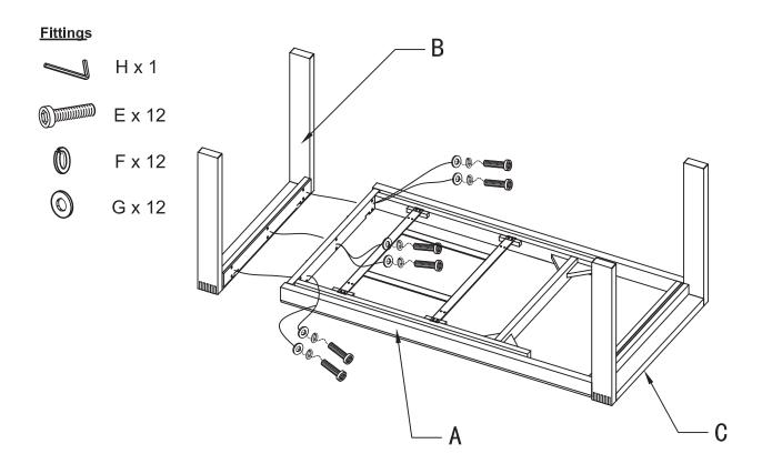
3. CAUTION this table is very heavy. With the aid of another person carefully lift the table and turn it over, taking care not to turn the table over on two legs as this may cause damage.
