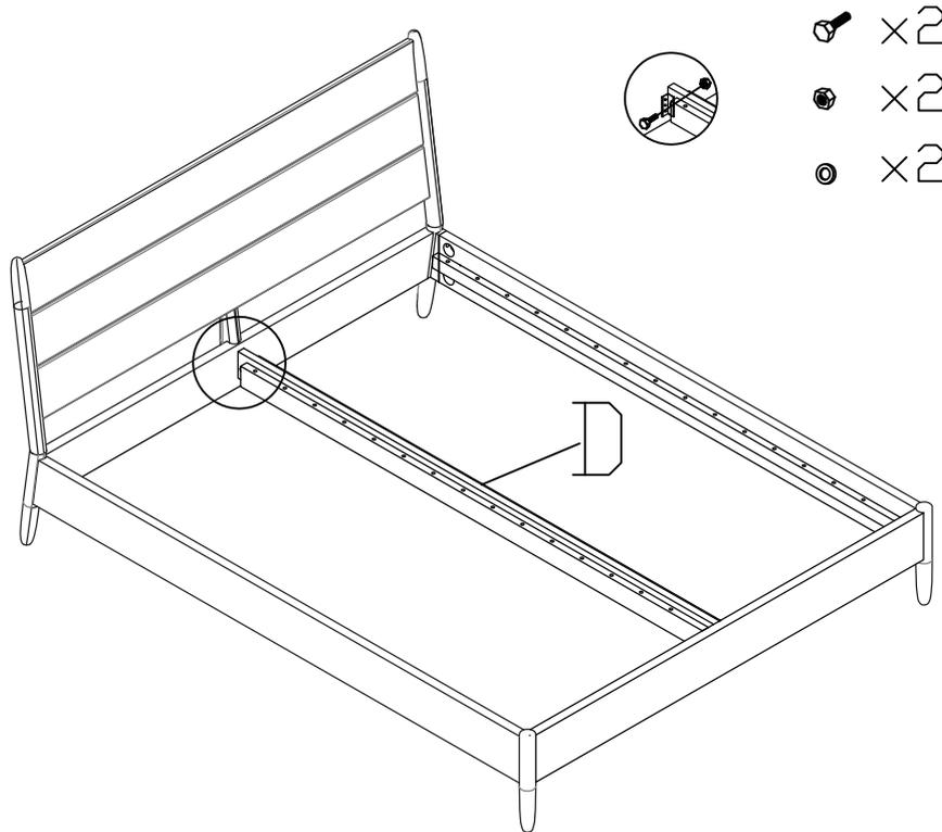
4. Push a plastic cap onto the end of each slat, ensuring that the peg is facing downwards, push the slat into the pre-drilled holes as shown below. Repeat for all of the slats. Assembly is then complete.
