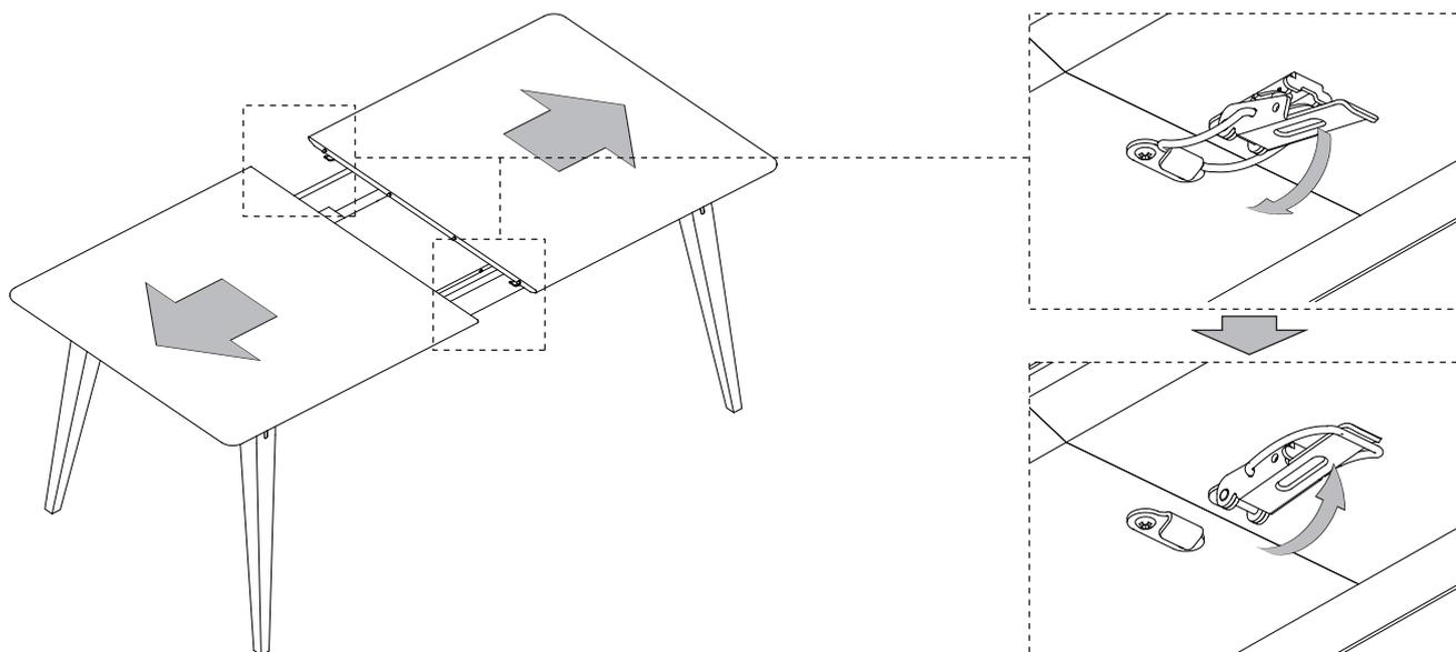
6. Take out the extension leaf and place it between the two halves of the top panel.
