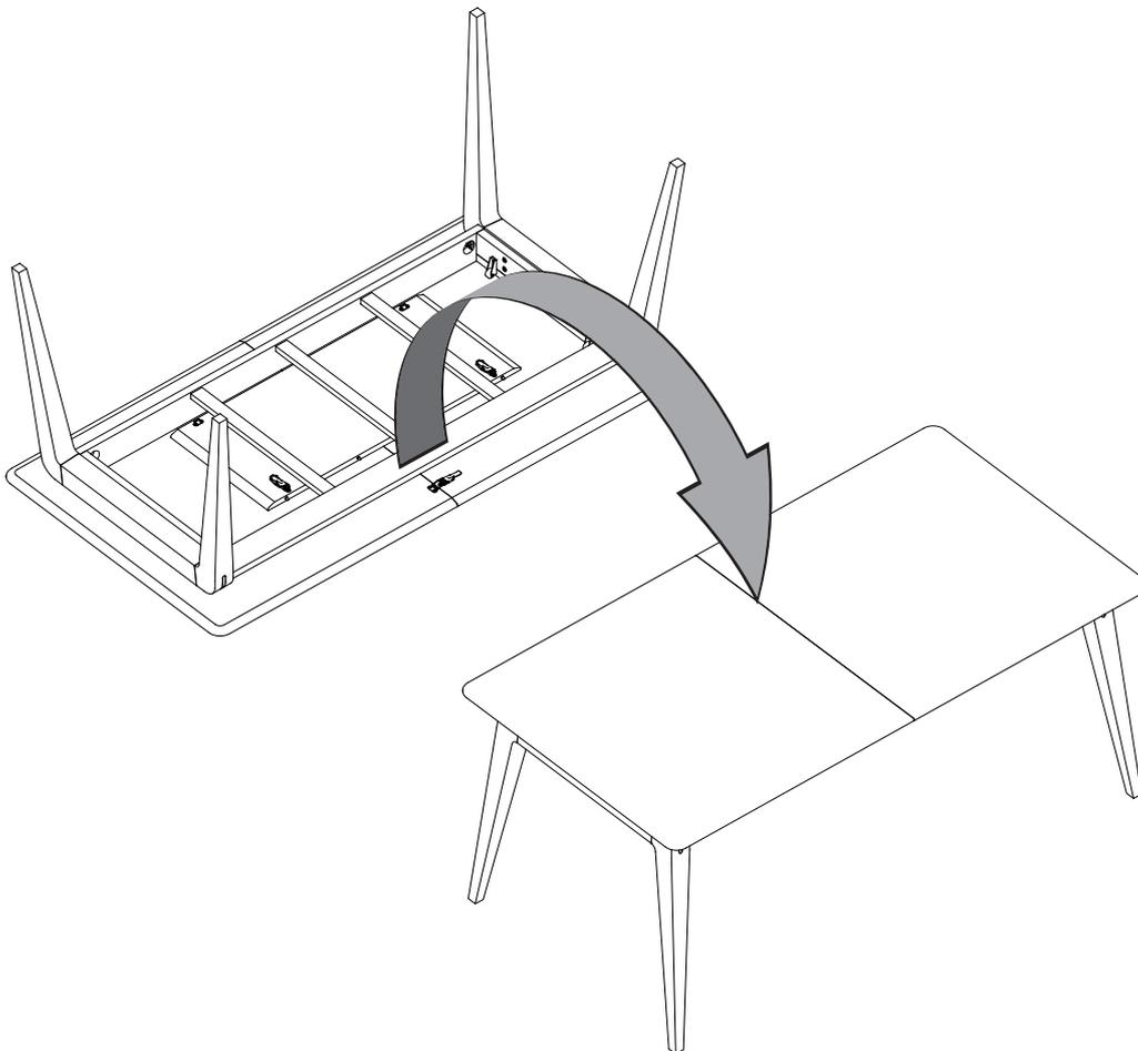
5. Release the two catch locks under the top panel and extend both halves.
