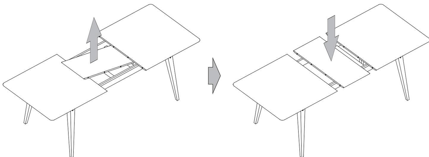
7. Fix the top panels in place by using the catch locks.
